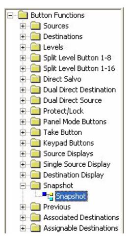
Snapshot buttons are used for defining a set of takes which can be triggered by pressing this button in the actual soft panel or retrieving a snapshot from the menu and taking it from there. These are only used with multiple destinations such as a monitor wall and are not to be confused with salvos. One or more of the outputs can be taken at the same time using a snapshot by retrieving the snapshot as a preset and then performing a take with the desired outputs by choice.
