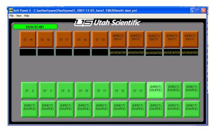
The cell in the upper-left corner should be green, indicating a successful connection to the controller. Red indicates a bad network connection between the SoftPanel's PC and the SC-4.
