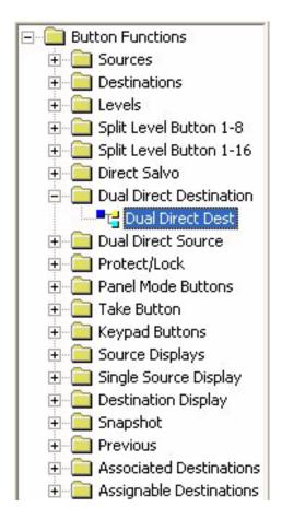
This allows a button to select the actual destination the panel will control. Assign (2) destinations to the button *after* assigning this function to the button. Once that happens, this button can be used to select the destination this panel will control.
