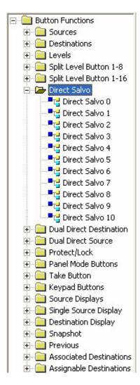
A Direct Salvo can be assigned to a button. To accomplish this, drag a "Direct Salvo #" and drop it on a button. When this button is pressed, it will send a command to the controller that will execute the direct salvo. The salvo must be configured in the SC4 *first* before this button will execute anything.
