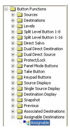
With this assigned as a destination button, the user can right click on the button in the panel to open the entire destination list of which they can select the desired destination.
