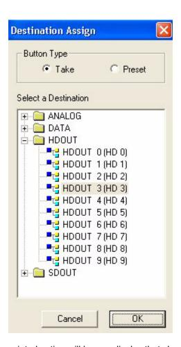
The associated option will have a display that shows the source status of what is switched to the assigned destination. The assignable option does not require a display. With either option there is also a source select that will bring up the source list of which the user may select from the entire list. NOTE: click the 'Take' item in the window to send that source directly to the destination. Otherwise, if 'Preset' is selected, then a Take button is required on the panel.
