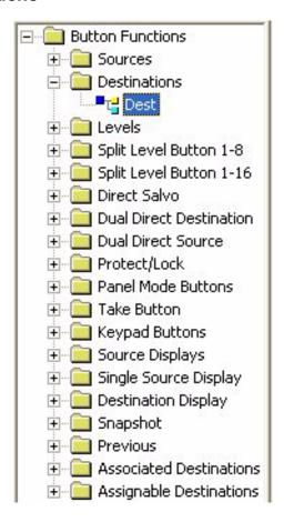
The Destination group will assign a button to control a given destination for this panel. The brightly lit destination is the current one that this panel will be switching *to*. If this panel does not contain any destination buttons, there should be a default destination assigned and labeled somewhere. In this way, the users can determine the appropriate output for this panel's control.
