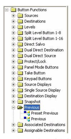
There are two options in the Previous folder. Both relate to reverting back to the previous switch after a take is made. This does not undo the current take but it literally goes back to the previous take made. The option called 'Preset Previous' shows the previous take in a blinking state before taking it, allowing the user the option to cancel or continue on with a Take. This mode also requires a Take button on the panel. The option called 'Previous' will perform the take without a prompt.
