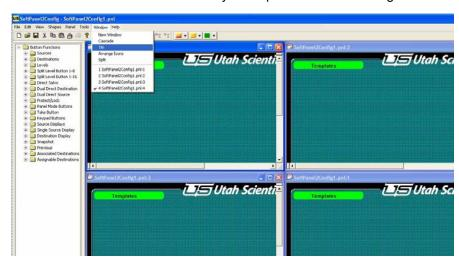
This is the 'Tile' view and will display the panels in a flat view all at once.
