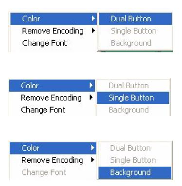
'Remove Encoding' – This option is used only with buttons and blanks out the selection that has been dropped onto that button. This does not include the functions but only the source and destination that is on the button. Another option for this instead of removing the encoding is to drag another source or destination on that button type.
