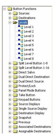
This type of level function is designed for simplicity and ease of use. If you assign a button as a "Level 1" through "Level 8" button, it functions in the following manner:
