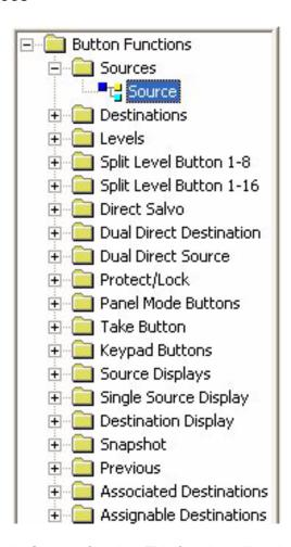
This is the Sources function. This function will assign the button to the Source Group. When this button is pressed a direct take will occur.
