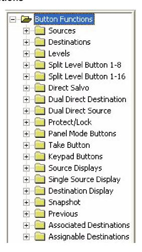
• The function menu has items that can be added to the various buttons and displays depending on how they are to be used.
